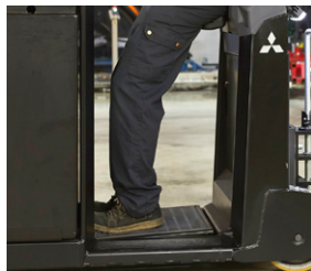
Suspended operator's platform.
