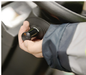
Steering directional control lever on the steering wheel (optional)
